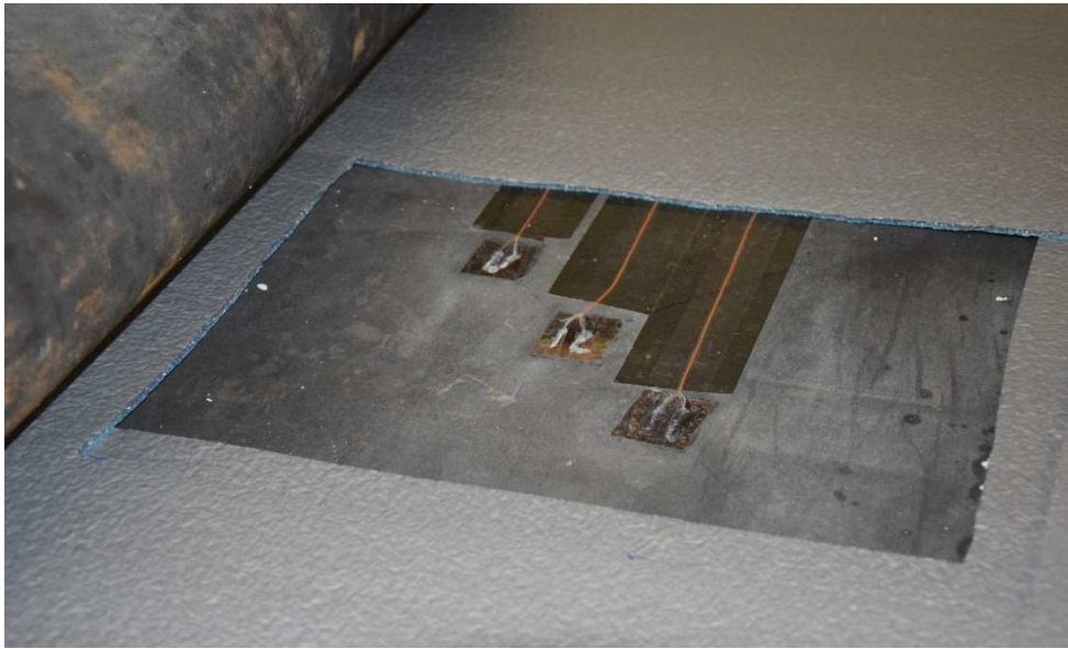
Figure 2.2. Sensors of the HFM apparatus for measurements of thermal conductivity
