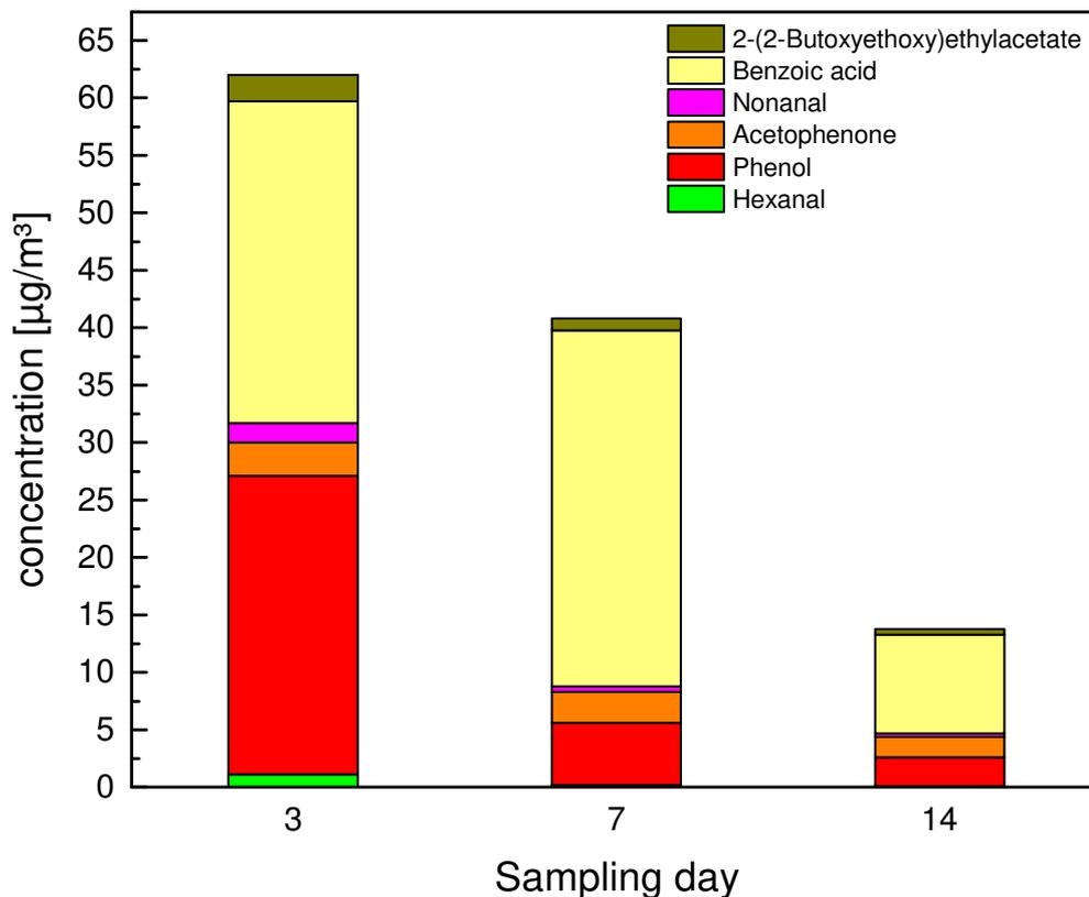
Figure 3.1 – Emission test results of NCC-foam sample
