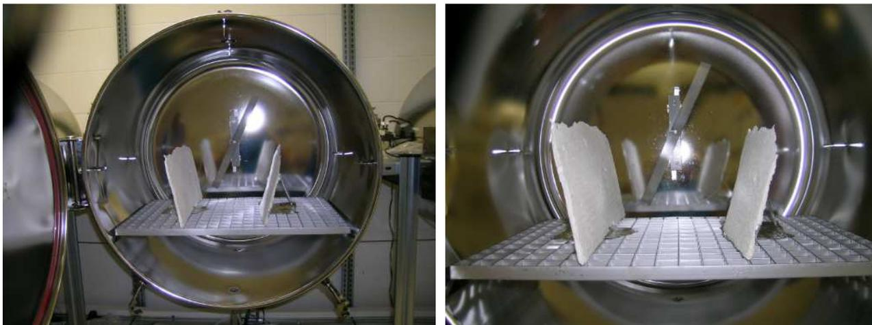
Figure 2.2 – Test chamber loaded with BRIMEE material
