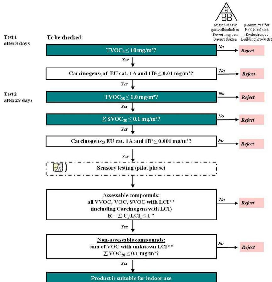
Figure 2.3 - Flow chart for the evaluation of VVOC, VOC and SVOC emissions from building products [6].
