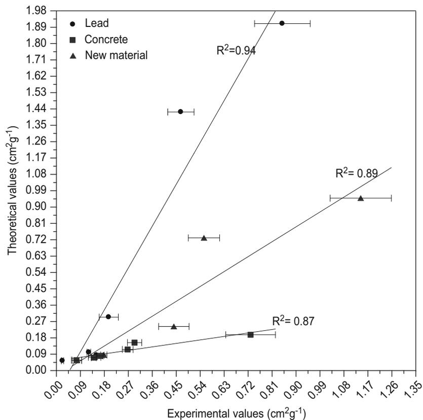
Fig. 3. The comparison of theoretical and experimental values of total mass attenuation coefficients.
