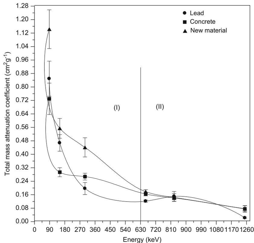
**Fig. 4.** The comparison of the experimental total mass attenuation coefficients for lead, concrete and the new material.
