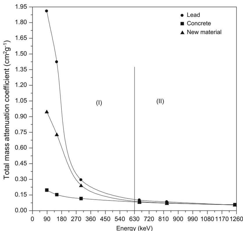
Fig. 5. The comparison of the theoretical total mass attenuation coefficients for lead, concrete and the new material.
